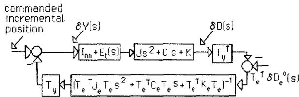
**Figure I-2:** The interaction of the manipulator and the environment when the target impedance is achieved for some bounded frequency range.
