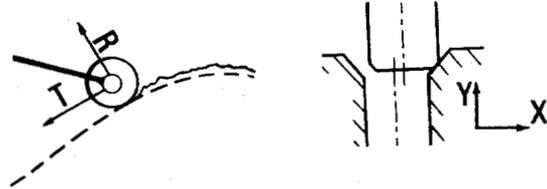
Figure 4-1 a: Grinding a Surface via a Manipulator, b: Peg in Hole
