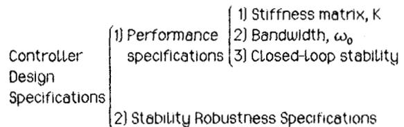
Figure 3-1: Controller Design Specifications
