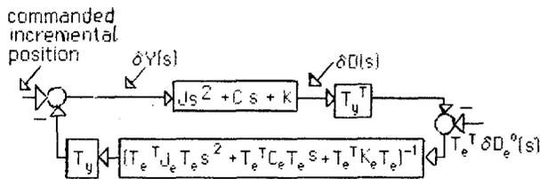
**Figure I-1** The interaction of the manipulator and environment in the ideal case when the target impedance is achieved for all  $0 < \omega < \infty$ .
