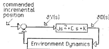
**Figure 5-1:** The interaction of the manipulator and the environment in the ideal case when the target impedance is achieved for all  $0 < \omega < \infty$ .
